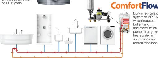
Built-in recirculation system on NPE-A2 which includes buffer tank and recirculation pump. The system heats water in supply lines via recirculation loop.
